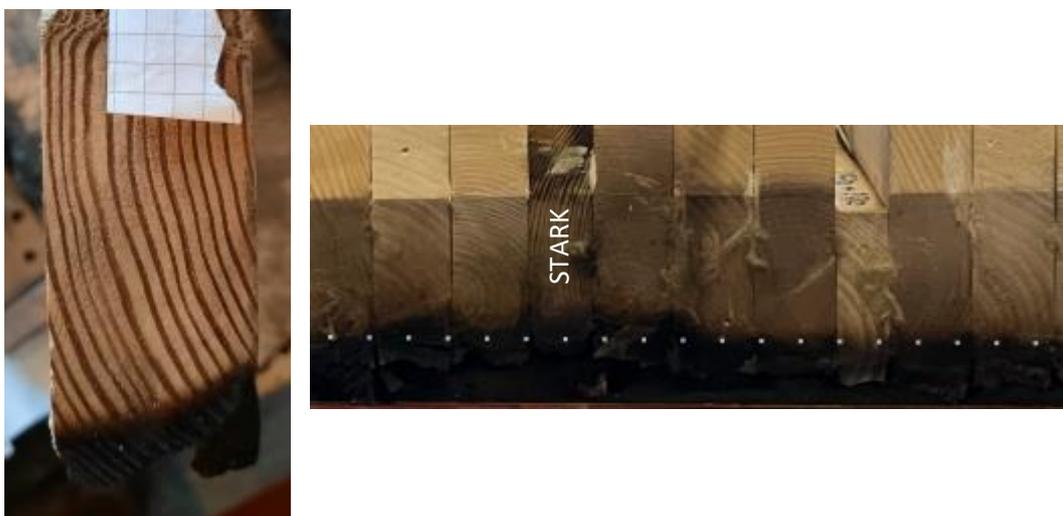
Figure 4. Char line of the Stark sample (left) and char line of whole specimen (right), with the Stark sample highlighted.
