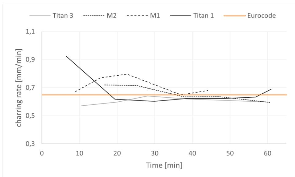
Figure 2. Charring rate during the fire test from the thermocouples measurements, including the 0.65 mm/min Eurocode rate.
