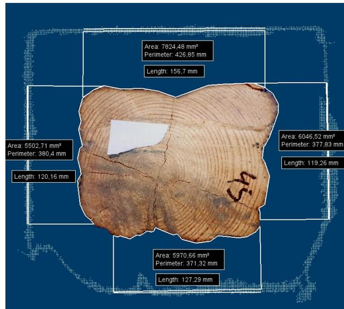
Figure 1. Example of measurements for the calculation of the charring rate of the Stark beam, with a non-square cross-section.
