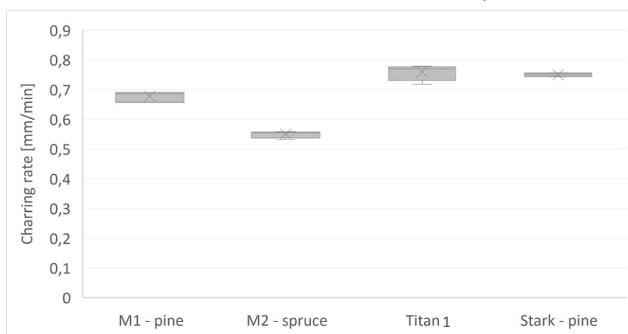
Figure 2. Charring rate distribution for each beam studied.
