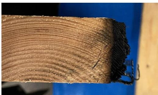
*Figure 5. Cut of sample M2, with a very flat char line.*
