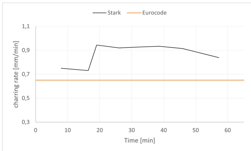
Figure 3. Charring rates of the Stark beam during the fire test, including the 0.65 mm/min Eurocode rate.
